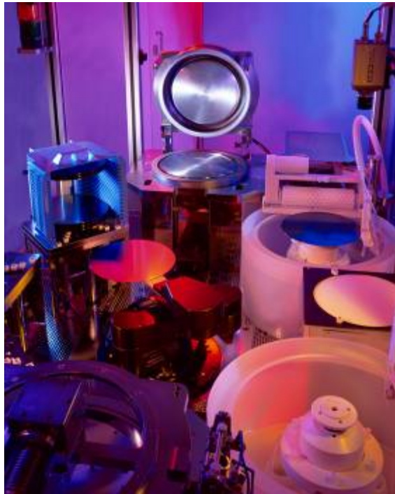
SiGen plasma-activation chamber (open chamber in background) integrated into an EV850 bond tool
