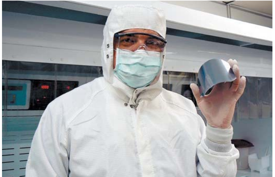
Francois Henley, director of production equipment manufacturer Silicon Genesis, with one of its ultra-thin wafers. The company bombards ingots with hydrogen ions to produce a silicon foil.
